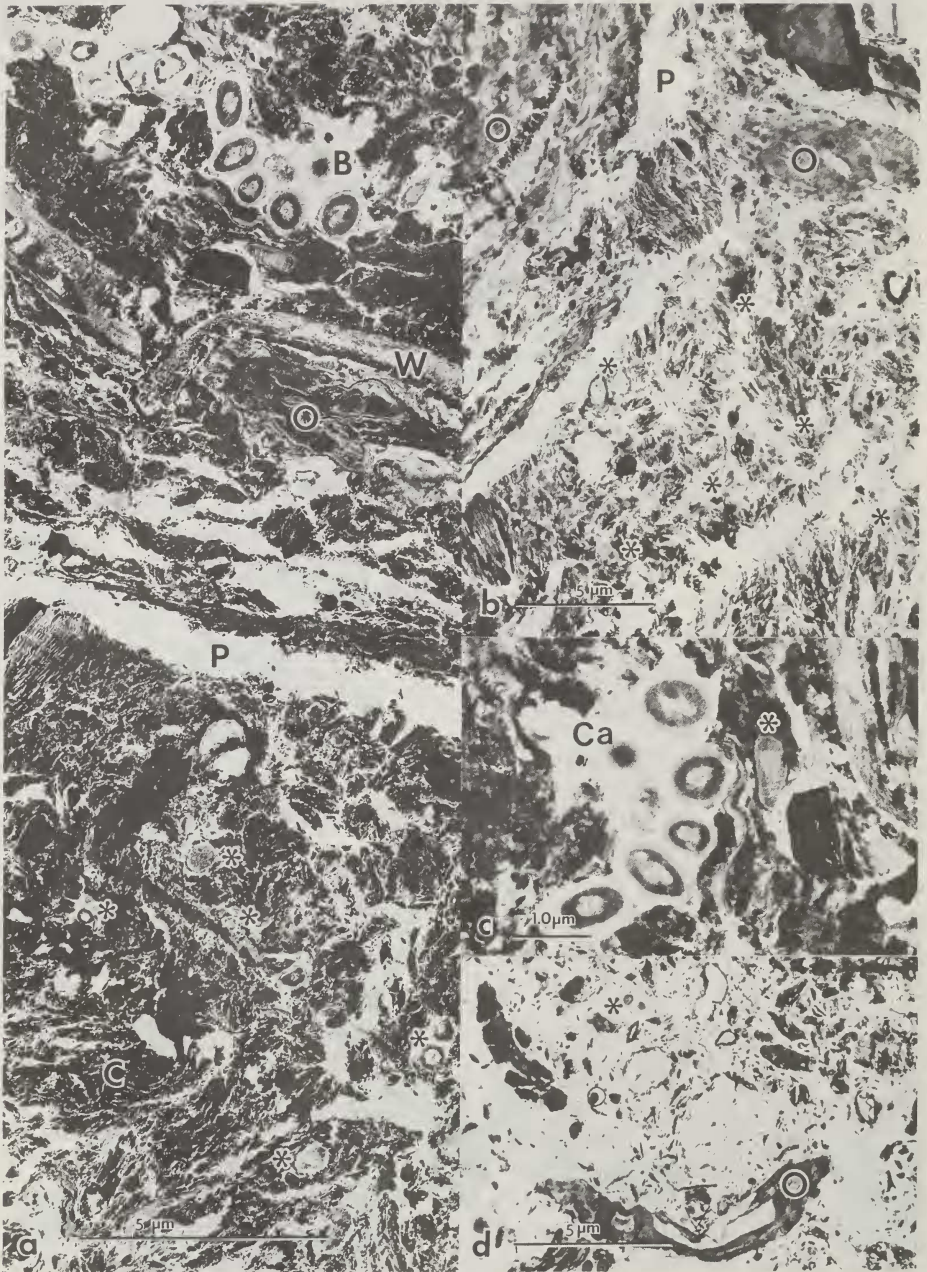
Plate 4. Soil fabrics with microorganisms and organic matter remnants.— (a). Bacteria (B) are usually associated with organic matter which still contains carbohydrate (eg. cell walls W). Other highly lignified and convoluted organic matter (O) does not support bacteria, but there are numerous microorganisms ( 0.3 \mu\text{m} diameter) scattered throughout the clay (*). P is a pore about 1 \mu\text{m} in diameter. (b). Similar to (a). (O) is amorphous organic matter. Again there are numerous small soil bacteria in the clay (*). (c). Detail of (a) showing bacteria enclosed in capsule material (Ca) which is not stained by Os04. (*) indicates a capsule-less bacterium enclosed in humified organic matter. (d). A less consolidated clay fabric containing remnants of cell wall remnants (O) and an occasional microorganism (*).
